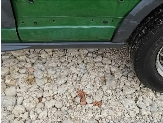
5: Qtr Panel Trim ns Missing Replace
