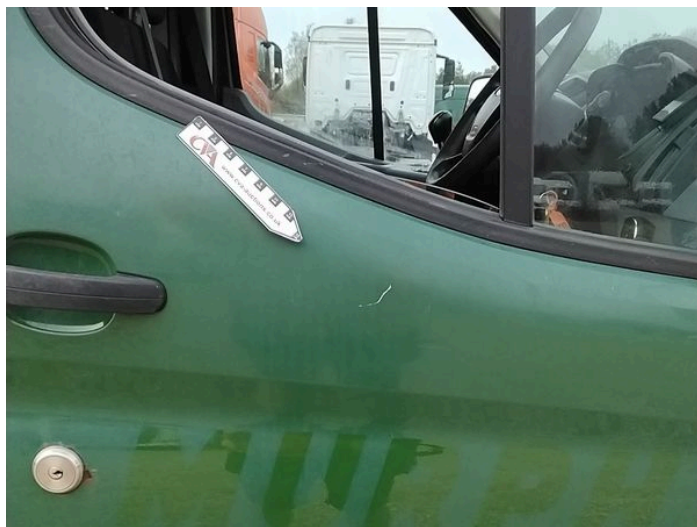
12: Door osf Scratched UpTo 25mm Thru Paint
