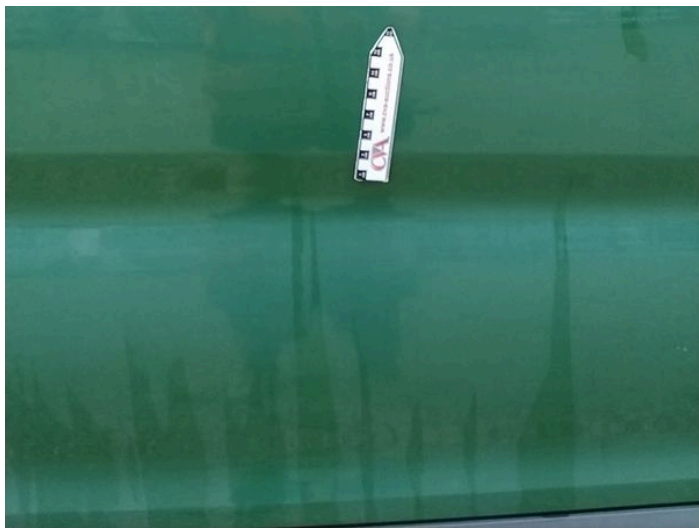
9: Qtr Panel osr Dented Over 2 UpTo 10mm
