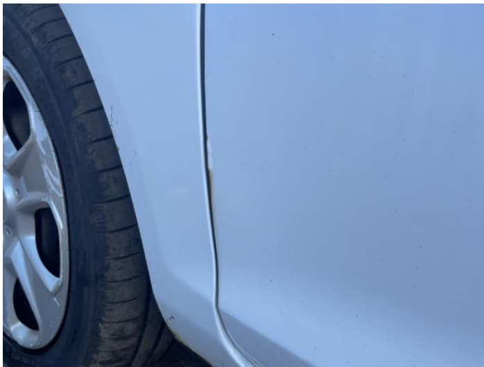
9: Door nsf Rusted UpTo 5mm
